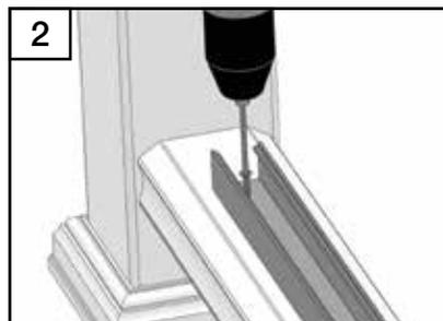
9. Center the top aluminum CVS rail, and secure using six of the supplied self drilling screws #10 x 1" (3 cm) (Figure 3).
